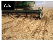
c. Whenever possible prior to installing the crop lifters on the header, combine approximately 100'/30m without the lifters to adjust the header angle, reel speed/height, header height, etc. to achieve optimal settings of the header alone. Once the lifters are installed, drive slowly over the path that has been harvested and observe whether or not the lifters need to be adjusted.
