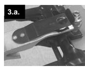
a. Slide the lifter snout over the guard with the rail spring side up. Push the lifter rail into the rail slot on the QD<sup>TM</sup> nut. The rail spring will pop into place under the safety groove. See Diagram 3 and 4.
