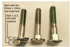
NOTE: Using the above configurations, the hexhead bolt may wear over time, in which case it will be difficult to remove without cutting or grinding it off. The hex-head may also catch plant material and rocks under the header.
